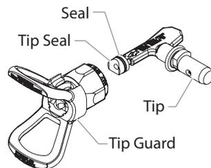
**NOTE: The arrow on the tip handle should be pointing in the forward direction for spraying.**
